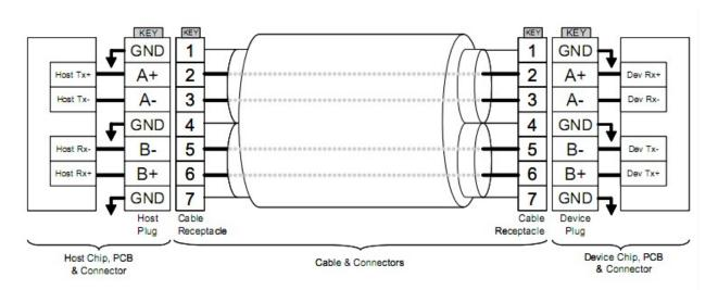
Figure 1-2 SATA Cable/Connector Connection Diagram
