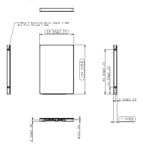
Figure 7-1 7mm Housing Physical Dimensions
