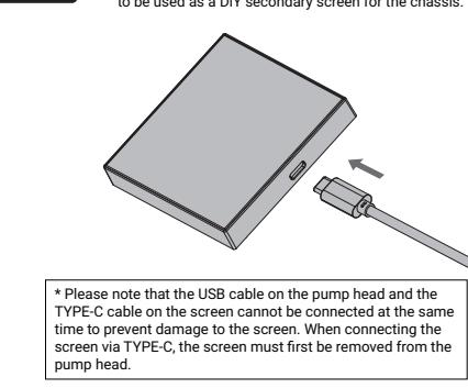
\* Please note that the USB cable on the pump head and the TYPE-C cable on the screen can not be connected at the same time to prevent damage to the screen. When connecting the screen via TYPE-C, the screen must first be removed from the pump head.
