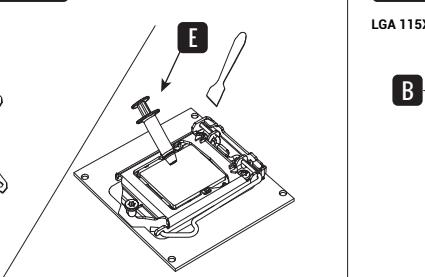
Remove the protection film / Applying thermal paste
