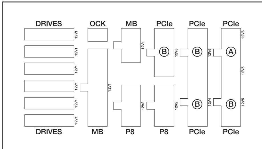
GPUs using 1 or 2 PCIe connectors = **(A)** | GPUs using >2 PCIe connectors = **(B)**
