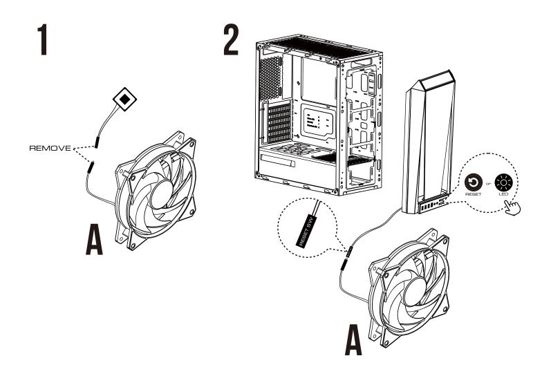
If your motherboard has 5V 3-Pin addressable (digital) RGB header, you can customize RGB lighting via motherboard manufacturer sync software
