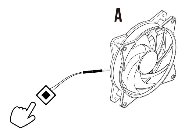
Two methods to control build-in RGB Lighting Method 2. If your case has "RESET SW", you can use case button to change lighting modes
