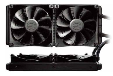
The EVGA CLC 280mm All-In-One RGB LED CPU Liquid Cooler has arrived! This new liquid cooler from EVGA gives you incredible performance, low noise, and robust software controls. The full copper waterblock pulls the heat from your CPU to the radiator, where newly designed fans, featuring Teflon Nano Bearings, effortlessly disperse the heat.
