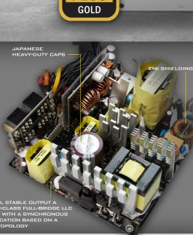
GOLD PRO WHITE series is tested for reliability and guaranteed to deliver up to 92% energy efficiency. 99% +12V OUTPUT
