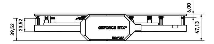
General tolerance: ± 0,25mm Dimension in millimeter
